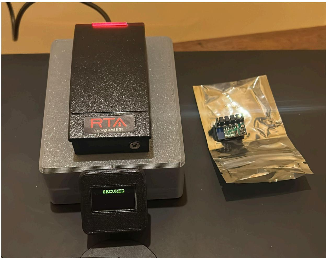
Above: Reader with ESPKey installed (left), and ESPKey on static-proof bag (right)
